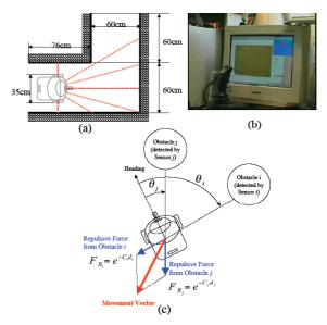
Figure 9. Testbed of tele-operated robot (a) task configuration (b) interface for a human (c) implemented machine agent's autonomy.
