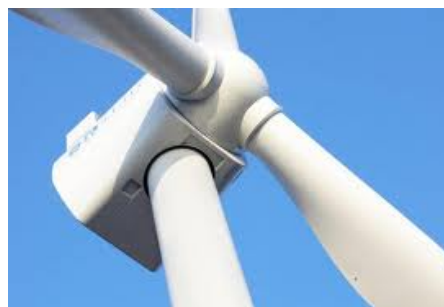
FIG 1. Big Glenn wind turbine located outside Gothenburg, Sweden. The turbine was manufactured by GE Wind Energy GmbH, and has rotor diameter 112.5 m with rated power of 4100 KW.
