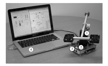
Fig. 1. Take-home helicopter set-up, showing (1) the 3-DOF helicopter, (2) signal conditioning and power electronics, (3) NI myDAQ interface, (4) PC running NI LabVIEW.
