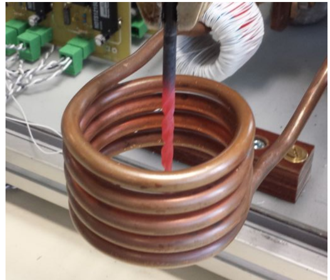
Fig. 4. A heating experiment: Work-piece at around 900^\circ\text{C} .
