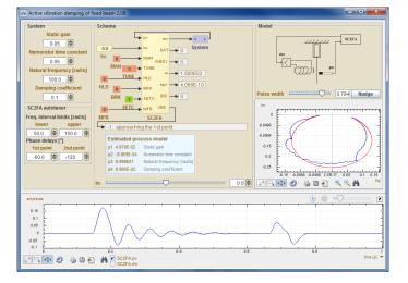
Fig. 2. SC2FA lab GUI – Advanced feedback vibration damping with autotuner
