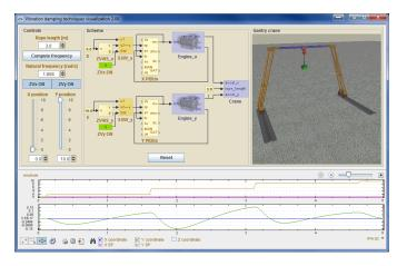
Fig. 4. ZV4IS lab GUI – Input shaping filter demonstrated on 3D gantry crane model
