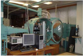
Fig. 7. SC2FA application – active damping of vibrating vanes in the wind tunnel
