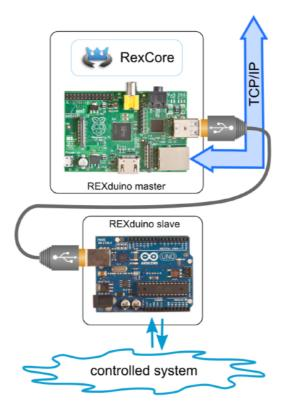
Fig. 8. Raspberry Pi + Arduino – the extremely low cost platform for running ContLab.eu algorithms in real-time
