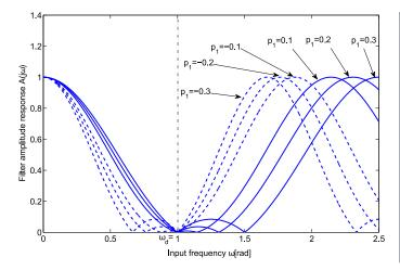
Fig. 3. ZV4IS – Influence of parameter  $p_1$  on the filter amplitude frequency response
