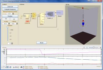
Fig. 5. ZV4IS lab GUI – Input shaping filter demonstrated on 3D spring-mass system model
