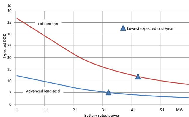
Fig. 6. Expected DOD and rated power of battery in simulation.
