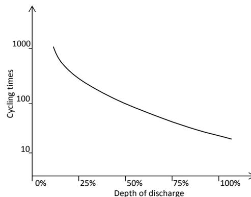
Fig. 1. Image of relation between DOD and life cycle by Liu et al. (2010).
