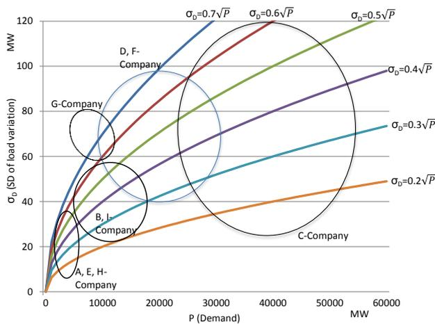
Fig. 2. Load variation characteristics for frequency control.
