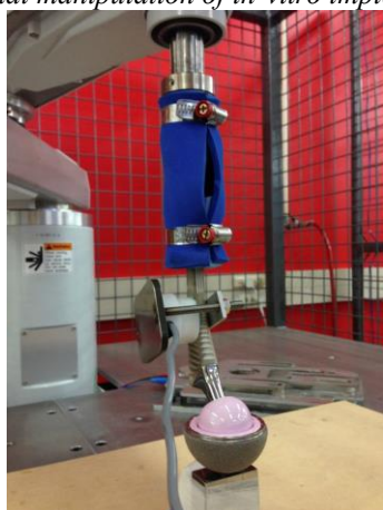
b) Automated robot manipulation of in-vitro implant testing
