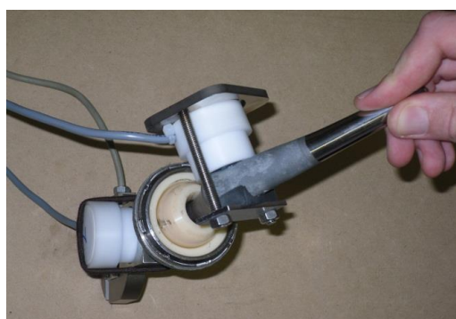
a) Manual manipulation of in-vitro implant testing
