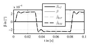
Fig. 7. System response and estimated system responses for observation with disturbance estimation
