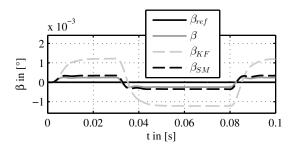
Fig. 5. System response in  $\beta$ -direction for ideal and observer based control without disturbance estimation
