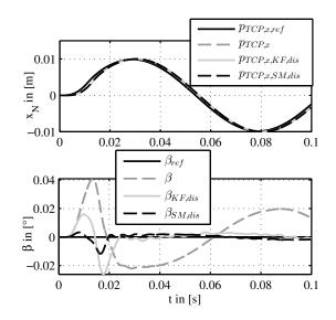
Fig. 9. System response for ideal and observer based control with disturbance compensation and MBS plant model
