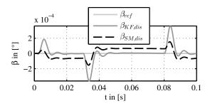
Fig. 8. System response in  $\beta$  direction for observer based control with disturbance compensation
