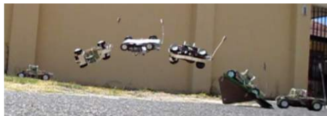
Figure 10: Actuated tail. FlipBot performing a complete 360 degree barrel roll
