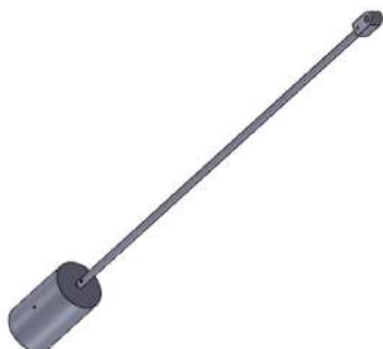
Figure 4: SolidWorks model of the tail was designed with an aluminium thread bar with a mild steel mass of 200g.
