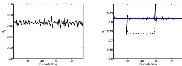
Fig. 4. Set point, state for the FTC (solid line) and state without FTC (dash-dot line) for the second fault
