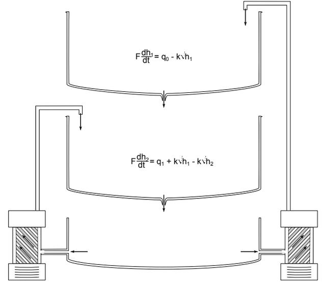
Fig. 1. Two-tank system
