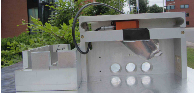
Fig. 3. Experimental setup where a calibration experiment is performed outdoors. An Xsens MTi-100 IMU (orange box) together with a magnetic disturbance is placed in a aluminum block.
