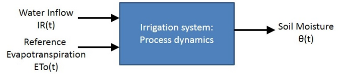
Fig. 3. Irrigation system input/output definition
