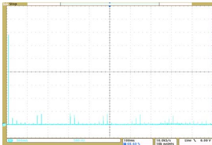
Fig. 19 Frequency spectrum of taken trolley current with zero vectors insertion
