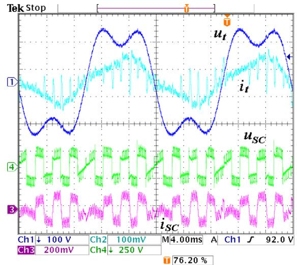
Fig. 11. The example of steady state under distorted power grid voltage
