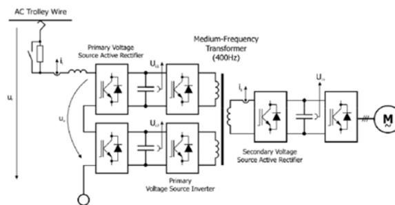
Fig. 2. Schematic diagram of the prototype vehicles with medium traction transformer and indirect frequency converter.
