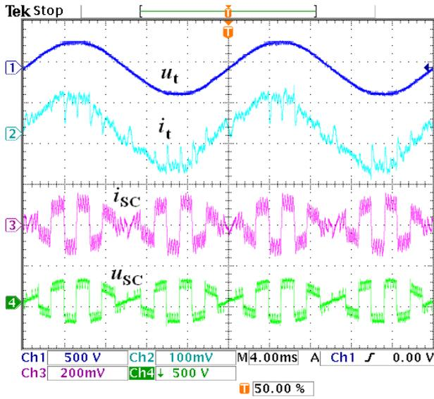
Fig. 7. Experimental results of traction drive with single matrix converter in rectifier mode
