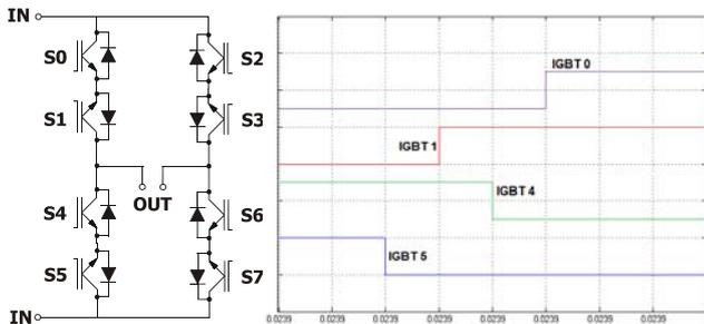
Fig. 4. Detail of matrix converter and 4-step commutation of matrix converter
