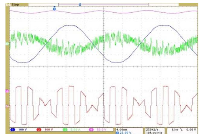
Fig. 17. Rectangular matrix converter control with zero vector insertion - inverter mode
