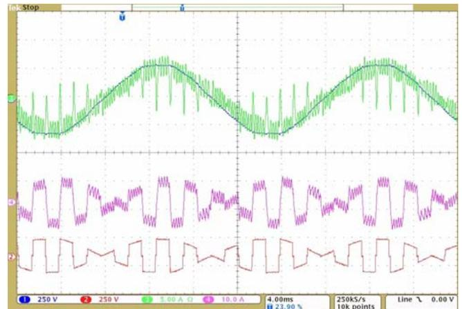
Fig. 16. Rectangular matrix converter control with zero vector insertion - rectifier mode
