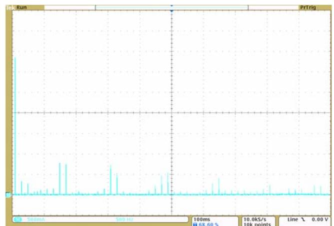
Fig. 18 Frequency spectrum of taken trolley current without zero vectors insertion
