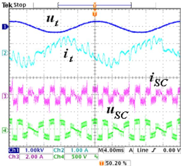
Fig. 8. Experimental results of traction drive with single matrix converter in inverter mode
