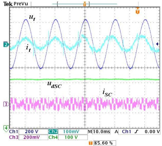
Fig. 9. Phase shift  $\varphi$  (between  $u_t$  and  $i_t$ ) change:  $0 - 45^\circ$ , rated power 2 kVA
