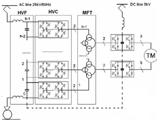
Fig. 3. Topology with single phase matrix converter as a primary high voltage traction converter.
