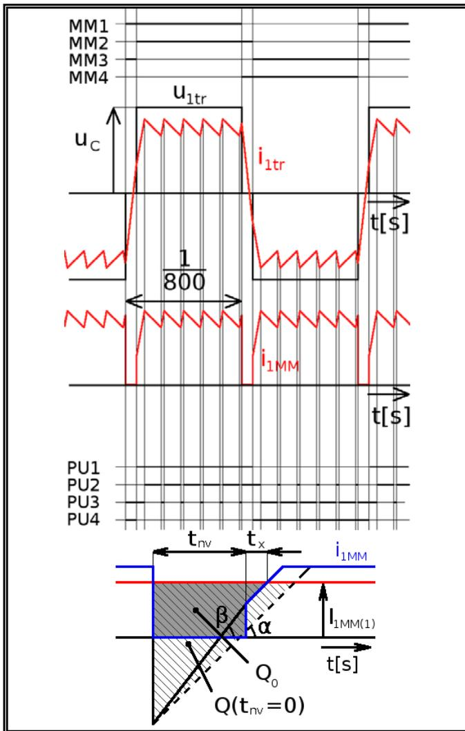
Fig. 15. Matrix converter current commutation with zero vector insertion (lower part - input matrix current, upper part - output matrix current)
