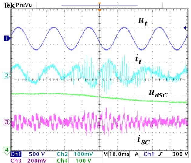
Fig. 10. Step change of  $U_{dSC}$ ,  $U_t=230$  V,  $P=2$  kW
