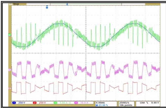
Fig. 12. Rectangular matrix converter control without zero vector insertion - rectifier mode
