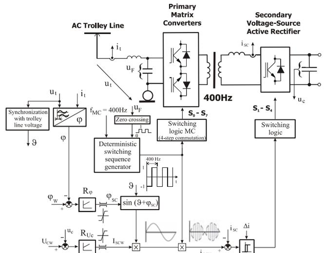
Fig. 6. Control algorithm scheme of the proposed traction drive
