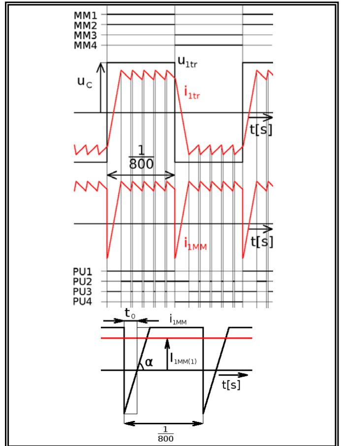
Fig. 14. Matrix converter current commutation (lower part - input matrix current, upper part - output matrix current)
