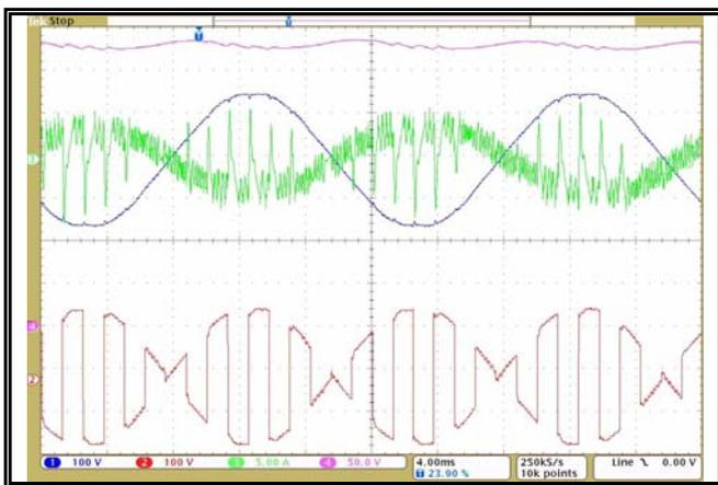
Fig. 13. Rectangular matrix converter control without zero vector insertion - inverter mode
