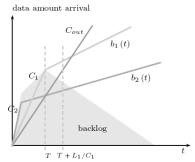
Fig. 2. Arrival and service curves and backlog evolution inside the two-input FIFO multiplexer.
