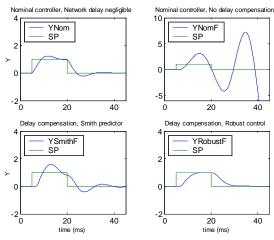
Fig. 8. The performance of the control system under various delay compensation strategies
