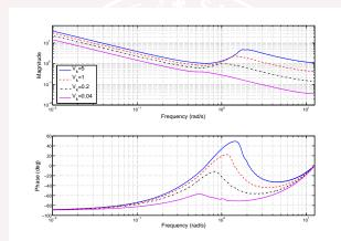
Prefered controller structure depends on desired trade-off between performance and control signal variance. Thus, a PI controller may very well be prefered over a PID.
