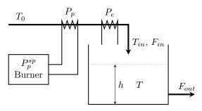
Figure 1. Tank with heated inflow.
