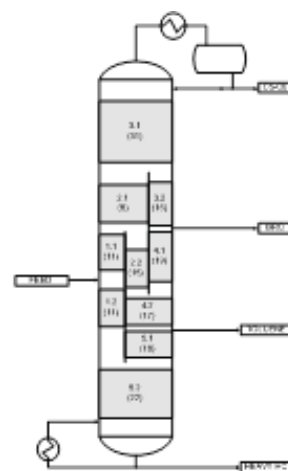
Figure 1. Four-product DWC with two partition walls.
