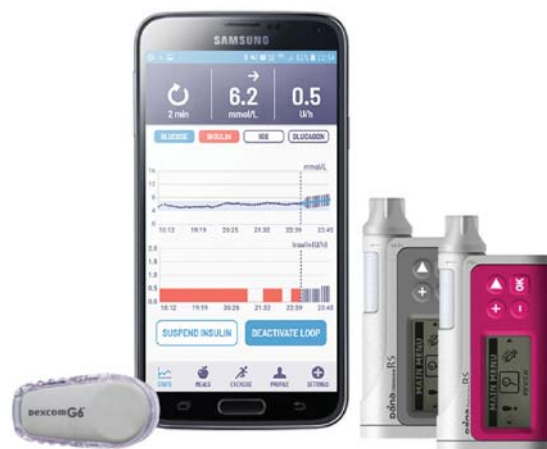
(c) Illustration of the AP prototype used in clinical studies. The glucose sensor is a Dexcom G6. Two Dana RS pumps are used to administer insulin and glucagon. The smartphone (Samsung Galaxy A5) is used to monitor the blood glucose concentration and previous injections of insulin/glucagon, to announce meals and to announce physical activity.
