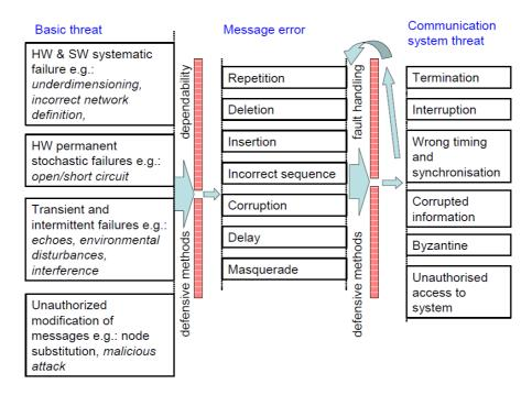
Figure 4: Fault model for wireless communications
