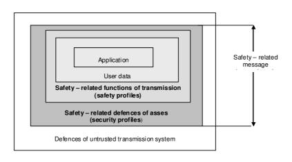
Figure 3: Model of safety - related communications in industrial applications
