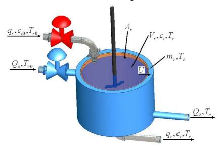
Figure 1: Continuous Stirred Tank Reactor (CSTR)
