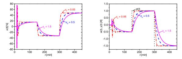
Figure 5: Course of input and output variables u(t) and y(t) for various weighting factors  $\phi_w$ , 1DOF configuration
