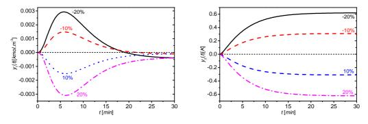
Figure 4: Dynamic analysis of outputs  $y_1$  ( $c_B(t) - c_B^s$ ) and  $y_2$  ( $T_r(t) - T_r^s$ ) for various step changes of the input heat removal,  $Q_c$
