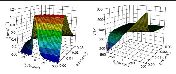
Figure 3: Steady-state values of the product's concentration,  $c_B^s$ , and the temperature of the reactant,  $T_r^s$ , for various heat removal,  $Q_c$ , and volumetric flow rate,  $q_r$
