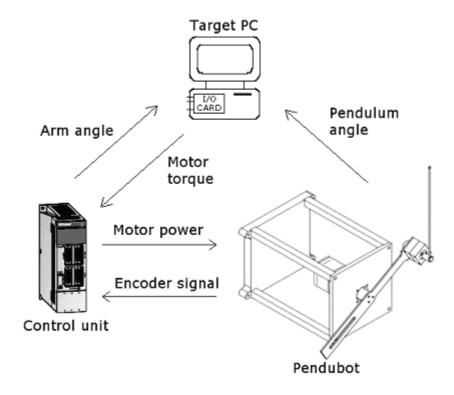
Figure 3: Pendubot hardware connection
