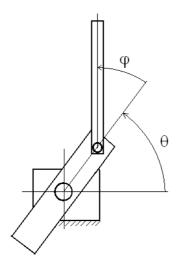
Figure 2: Measured angles
