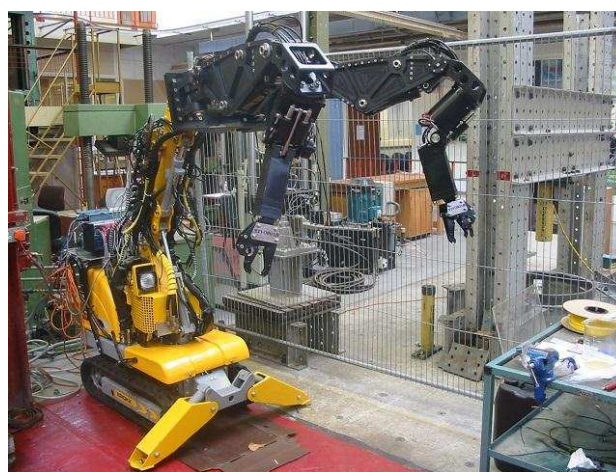
Fig. 1. Brokk-40 and dual HydroLek-7W manipulators.
