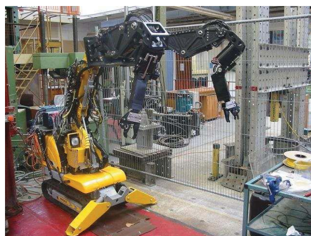
Fig. 1. Brokk-40 and dual HydroLek-7W manipulators.
