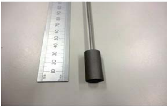
Figure 5: Incorporation of mini HTFP ingot with a metal sheathed tungsten rhenium (W-Re) thermocouple [15].
