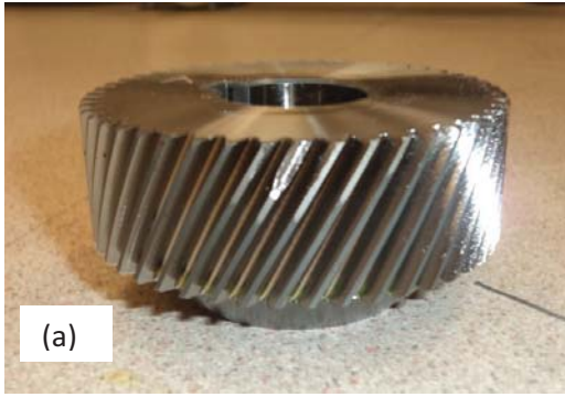
Figure 2: (a) Gear No 7 with 25% tooth breakage (Baseline)
