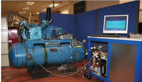
Figure 1 Reciprocating compressor test system.
