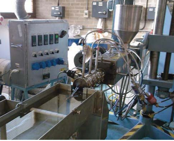
Fig. 2: The laboratory extruder with a in-line-rheometer die
