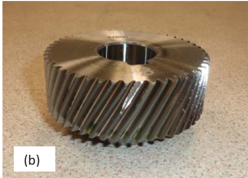
(b) Gear No 8 with 50% tooth breakage
