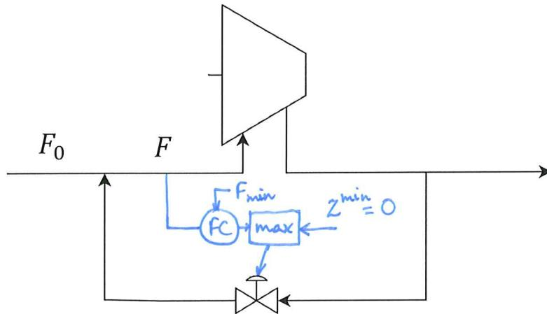
In this system, the compressor must be fed a minimum flow  $F \geq F_{min}$  in order to avoid abnormal operation. However, the system should also operate with the recycle valve fully closed whenever possible, in order to avoid additional compression costs. The process feed  $F_0$  is the main disturbance for the process, and the recycle valve is the only available MV.
