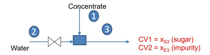
You are mixing two streams. Stream 1 contains water (W), sugar (S) and some preservative (E). Your task is to mix the feed (stream 1) with pure water (stream 2) to get a product (stream 3) that satisfies:
