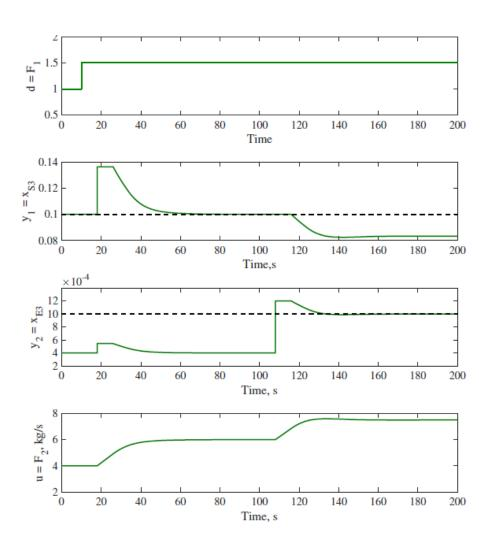
Figure 10: Simulation results for a step disturbance  $F_1 = 1.5 kg/s$  at t = 10 s and  $x_{E1} = 0.006$  at t = 100 s (extreme case). The black dotted lines show the concentration specification for  $x_{S3}$  and  $x_{E3}$  respectively. In the normal case, the controller is controlling  $y_1 = x_{S3}$  at  $y_{1s} = 0.1$ , while in the extreme case, the controller is controlling  $y_2 = x_{E3}$  at  $y_{2s} = 0.001$ .
