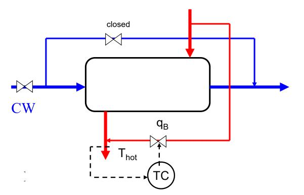
Use "dynamic" input  $q_B$ Advantage: Very fast response (no delay) Problem:  $q_B$  is too small to cover whole range + has small steady-state effect
