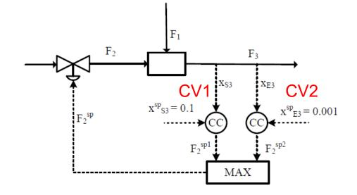
Figure 9: Control structure that handles both the nominal and the extreme cases
