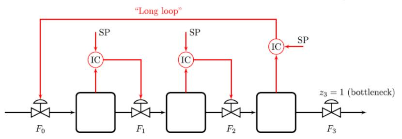
(d) Inventory control with undesired "long loop", not in accordance with the "radiation rule" (for given product flow, TPM=  $F_3$ )
