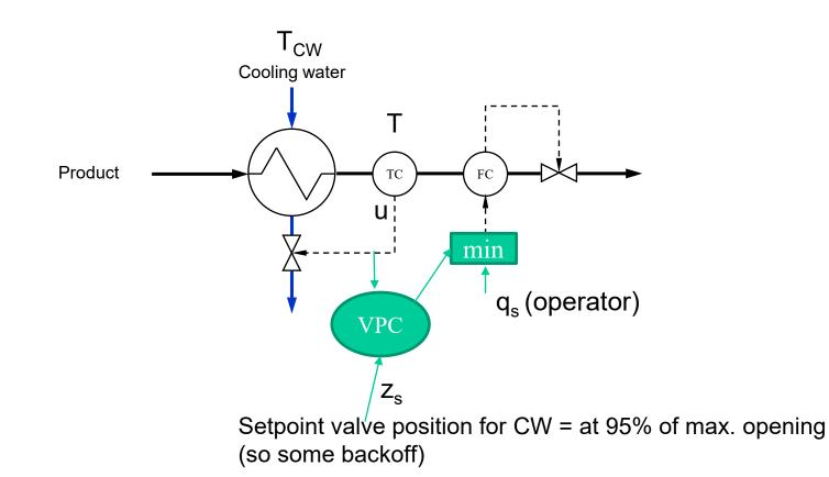
Comment: 1. Has the advantage of not changing the controller for T. 2. With  $q_s$  large (infeasible setpoint) one can have q=qmax (as long as  $q_{CW}$  < max) 3. But cannot quite achieve fully open CW valve (so some loss = backoff)
