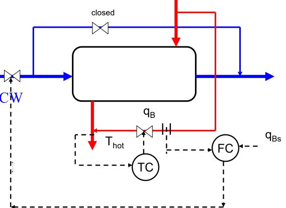
TC: Gives fast control of  $T_{hot}$  using the "dynamic" input  $q_B$ FC: Resets  $q_B$  to its setpoint (IRV) (e.g. 5%) using the "primary" input CW
