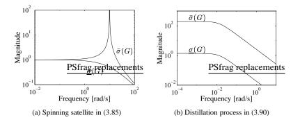
Figure 3.6: Typical plots of singular values
