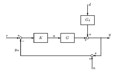
Figure 3.7: One degree-of-freedom feedback control configuration
