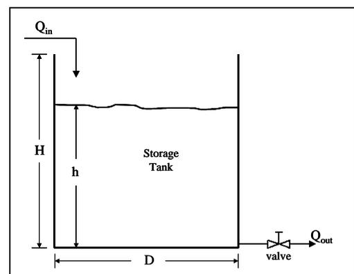
fluid level inside the tank is  $h$  (m). Fluid is flowing into the tank at rate  $Q_{in}$  ( $m^3/s$ ). Fluid is flowing out of the tank through an outlet valve at rate  $Q_{out}$  ( $m^3/s$ ). The question is what is the fluid level,  $h$ , as a function of time?
