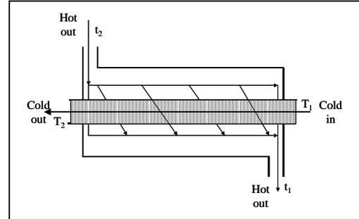
The design equation for counter-current heat exchange is
