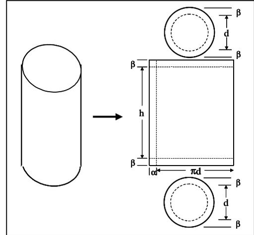
The objective in can design is to use the minimum amount of material to enclose a specified volume. The volume enclosed by a right circular cylinder is
